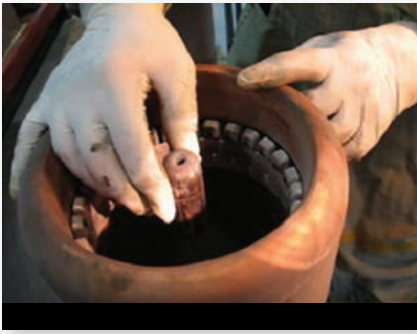
Fig. 5. Unscrewing of tungsten tip.
