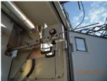
With a resistive displacement transducer Ref : ZRT-01/03/05/10
