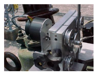
With a our KIT-ZLR linear-to-rotary motion converter and a ZRT-05 rotary transducer.
