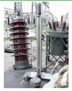
With a KIT-ZLB linear kit and a ZLT-600 linear transducer.
